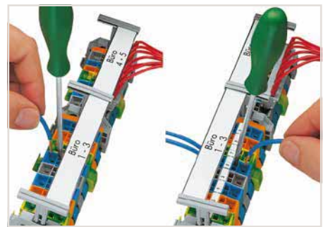
Sliding marking strips laterally.
