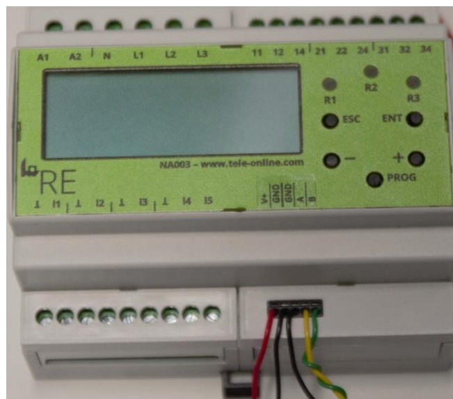
Figure 8: Exemplary connection Modbus interface NA003.COM
